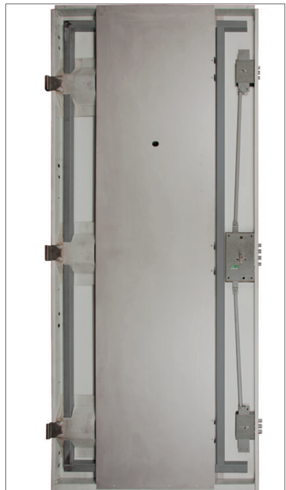
6- Reinforced chassis 35x35x2 mm inside the frame. It serves to give stiffness to the armored door and to preserve the closure points at the moment of forcing.
