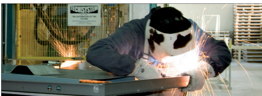
Welding of the door body.
