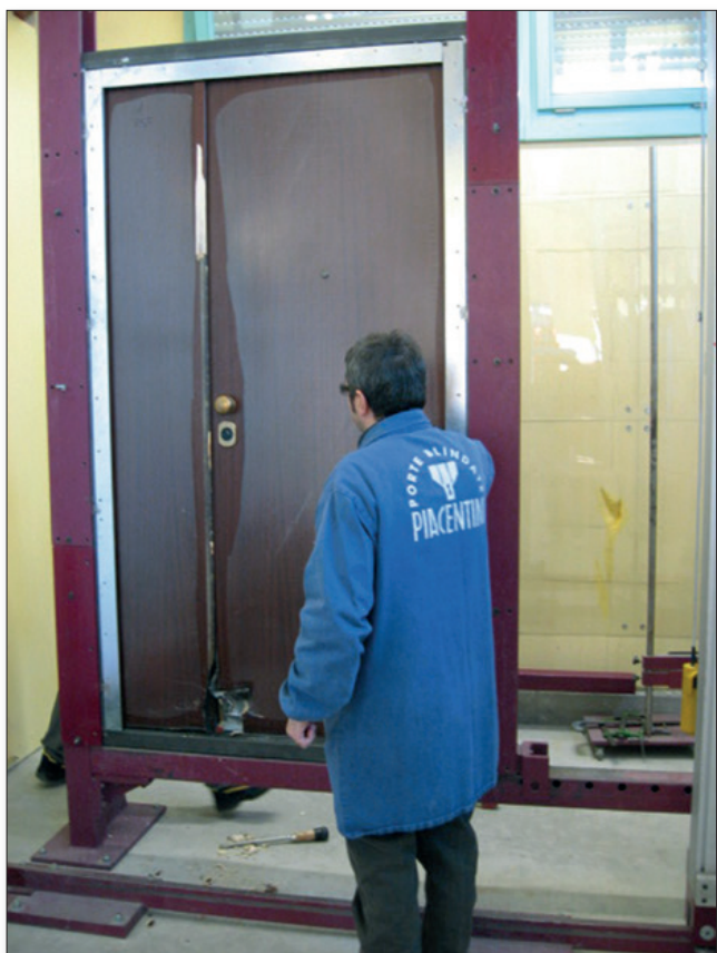
Anti-burglary: manual attack test.
