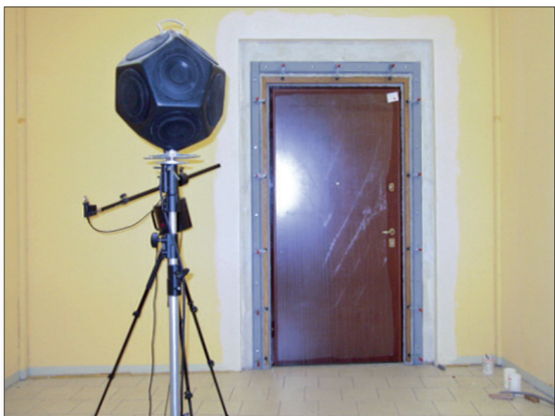
Acoustic isolation test.
