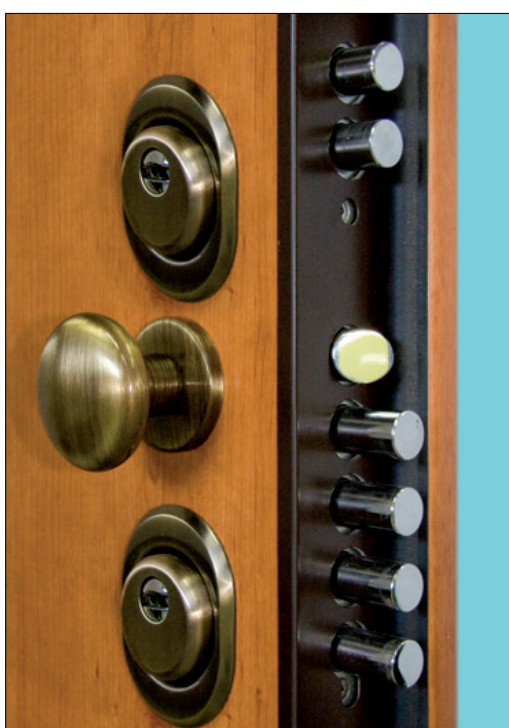
EUROPEAN LOCK 28/63 gear with LOCK SERVI- CE, controls the two upper bolts and the latch, blocks the main lock.
